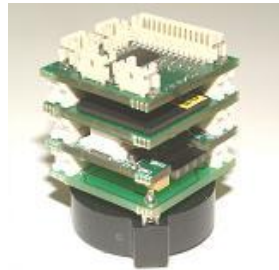
Fig. 1. 25mm prototype module with coin battery
