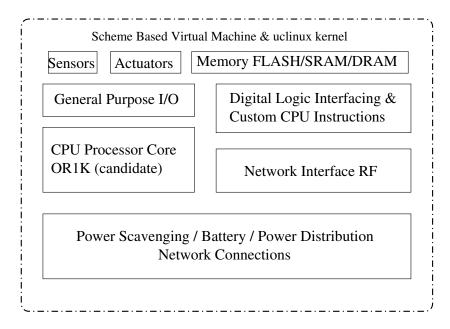
Fig. 1. Proposed target architecture.
