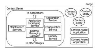
Fig. 1. The set of components which make up ConStruct.
