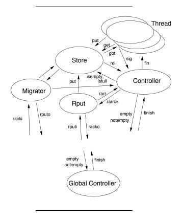
Fig. 4. Global system of agents, extending the local system to facilitate termination detection across multiple address spaces.
