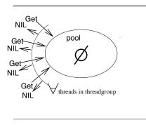
Fig. 2. Multiple processes accessing an empty pool data structure, with consensus termination detection.
