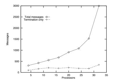
Fig. 5. Termination message count against total message count within a distributed implementation of a weakly coherent priority queue. Figures obtained from usage inside a branch-and-bound parallel solver averaged over several executions of a set of benchmark problems.
