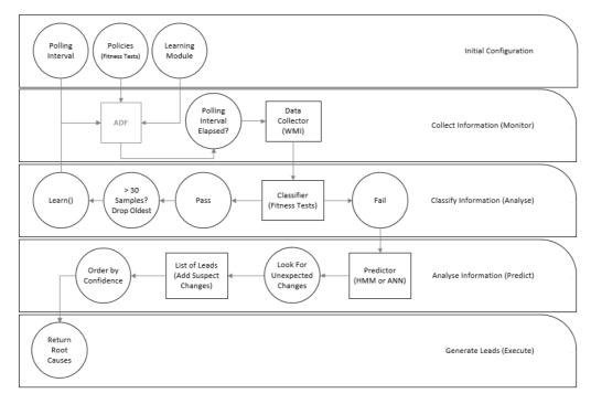
Figure 1: Anomaly Detection Framework Logic & Architecture Diagram
